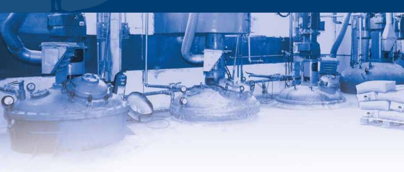
olvent based adhesive manufacture has been the initial production type from the foundation of the company. Today, Oynurden has the largest production capacity of solvent based adhesives in Europe. At the moment 10000 tonnes/year. of different types of solvent based adhesives can be produced with the fully closed-circuit system. To realize this capacity level, custom made, computerized continuous filling systems are being operated.
